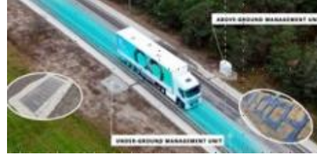
The two technologies to be integrated in A 10 close to Longvilliers, ground conductive (left view) and inductive (right view)
